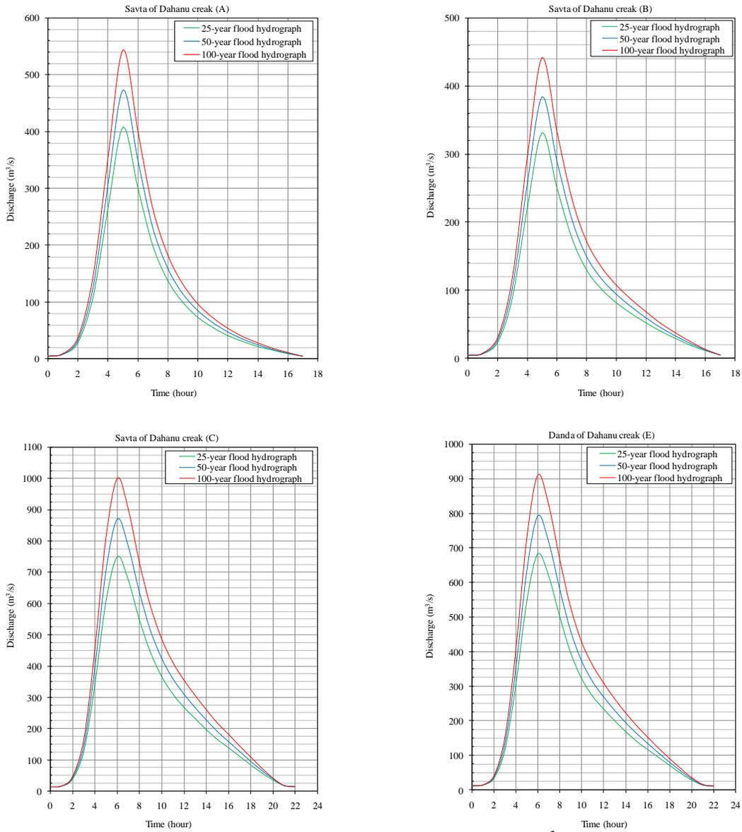
Figure 6. Flood hydrographs for the ungauged catchments with catchment area more than 25 km<sup>2</sup> in the study area of VPP
