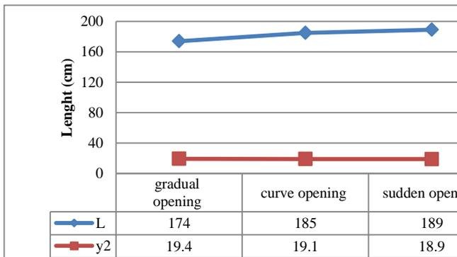
Figure 9. Graph of secondary jump length and depth at a flow rate of 41.4 l/s.
