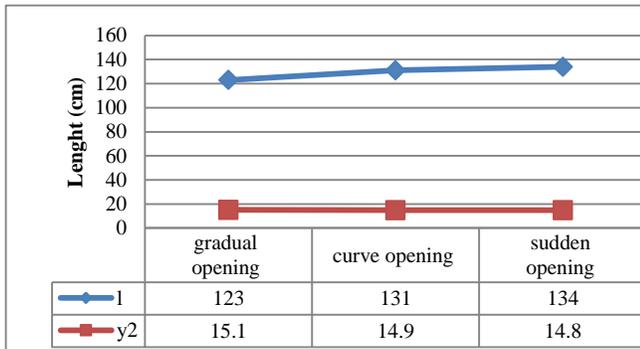
Figure 8. Comparison diagram of secondary jump length and depth at a flow rate of 27.4 l/s.
