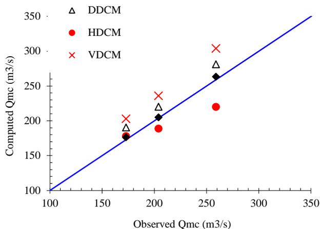
**Figure 5.** Predictions of the traditional divided channel methods and GEP model for main channel flow discharge (River Severn at Montford Bridge)
