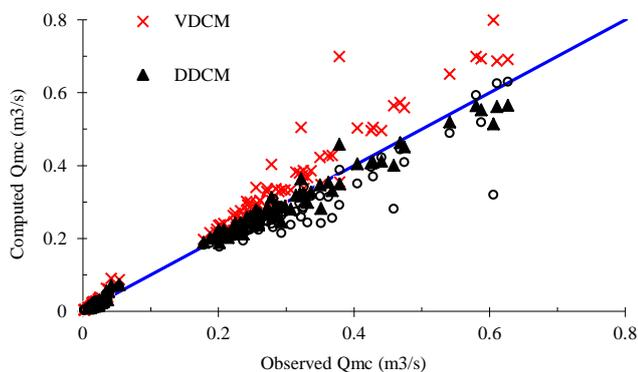
**Figure 3.** Flow discharge calculation of traditional divided channel methods for main channel
