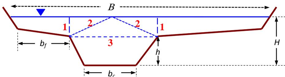
**Figure 1.** A compound river channel with common dividing channel methods, 1: vertical, 2: diagonal and 3: horizontal dividing models
