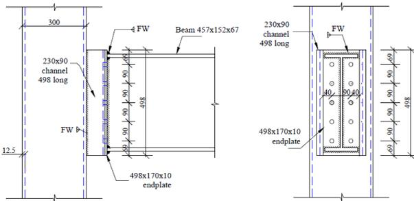
Figure 8. Connection with balanced endplate
