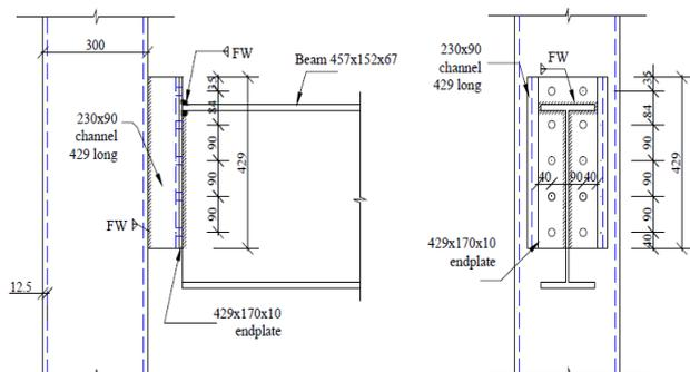
Figure 11. Connection with flexible extensive endplate
