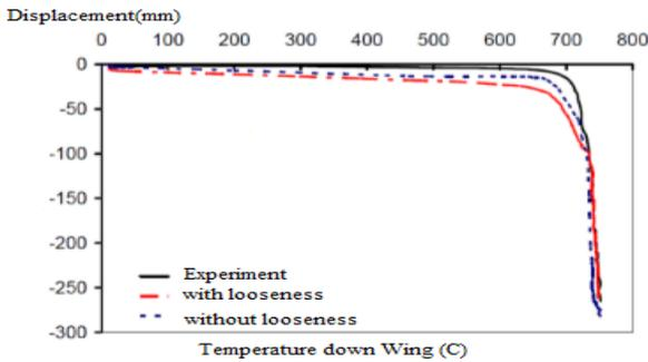
**Figure 18.** Comparison of beam displacement with looseness of different screw
