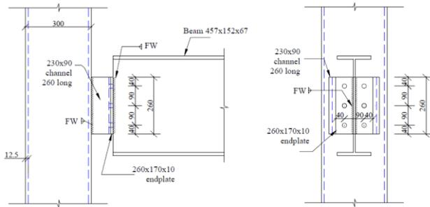
Figure 7. Connection with flexible endplate
