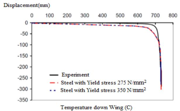
Figure 16. Comparison of beam displacement with different yield stress
