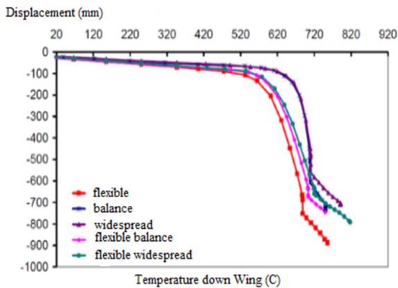
**Figure 22.** Comparison of displacement in the middle of beam span in connections with various endplate
