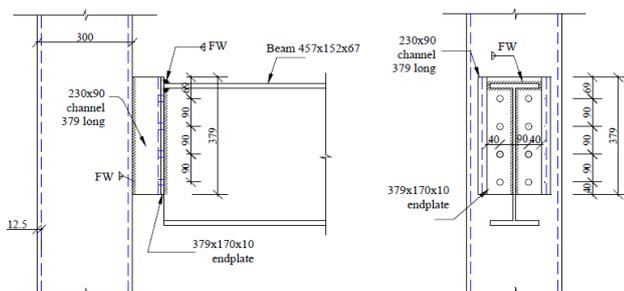
Figure 10. Connection with flexible balanced endplate
