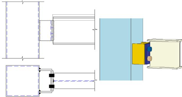
**Figure 1.** Reverse channel connection with flexible endplate
