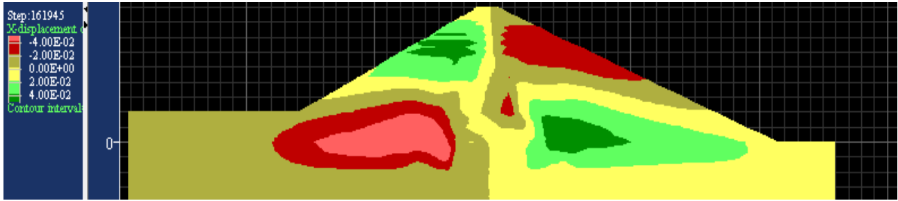
Figure 3. Horizontal deformation after construction
