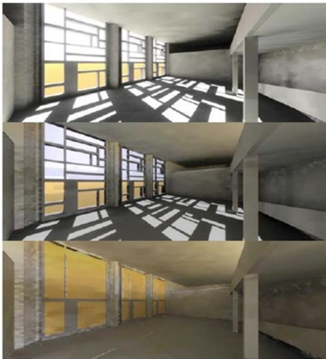
Figure 7. Interior spaces of the SE of The Kuwaiti National Museum with different glazing systems: (top) existing conditions, (center) switchable glazing, and (bottom) switchable glazing with dynamic louvers and motorized shading. (Source: Beltrán, 2003)]
