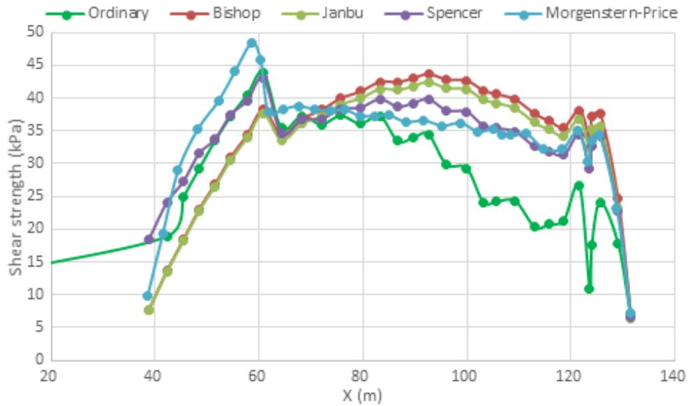
**Figure 11.** Comparisons between the determined resisting forces on failure surface.
