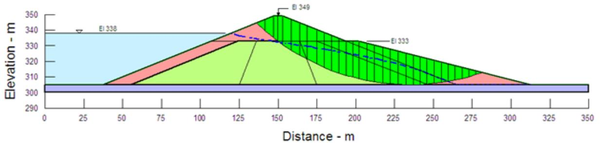
Figure 7. Critical failure surface of earth dams downstream
