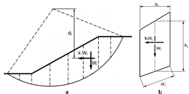
Figure 3. (a). Slope with weight and seismic forces, (b). Dimensions for an individual slice
