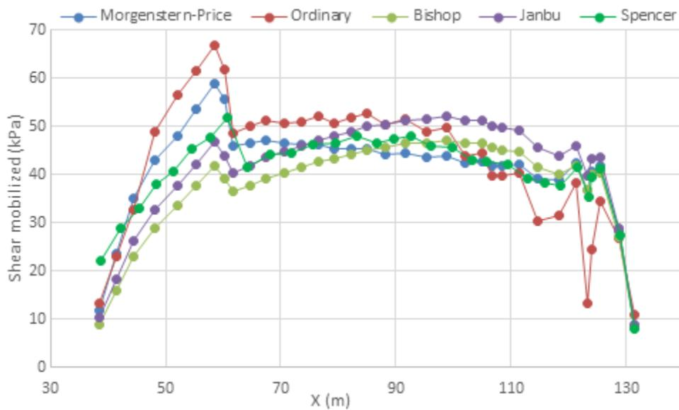
**Figure 12.** Comparison of the driving force in the pieces leg by various methods
