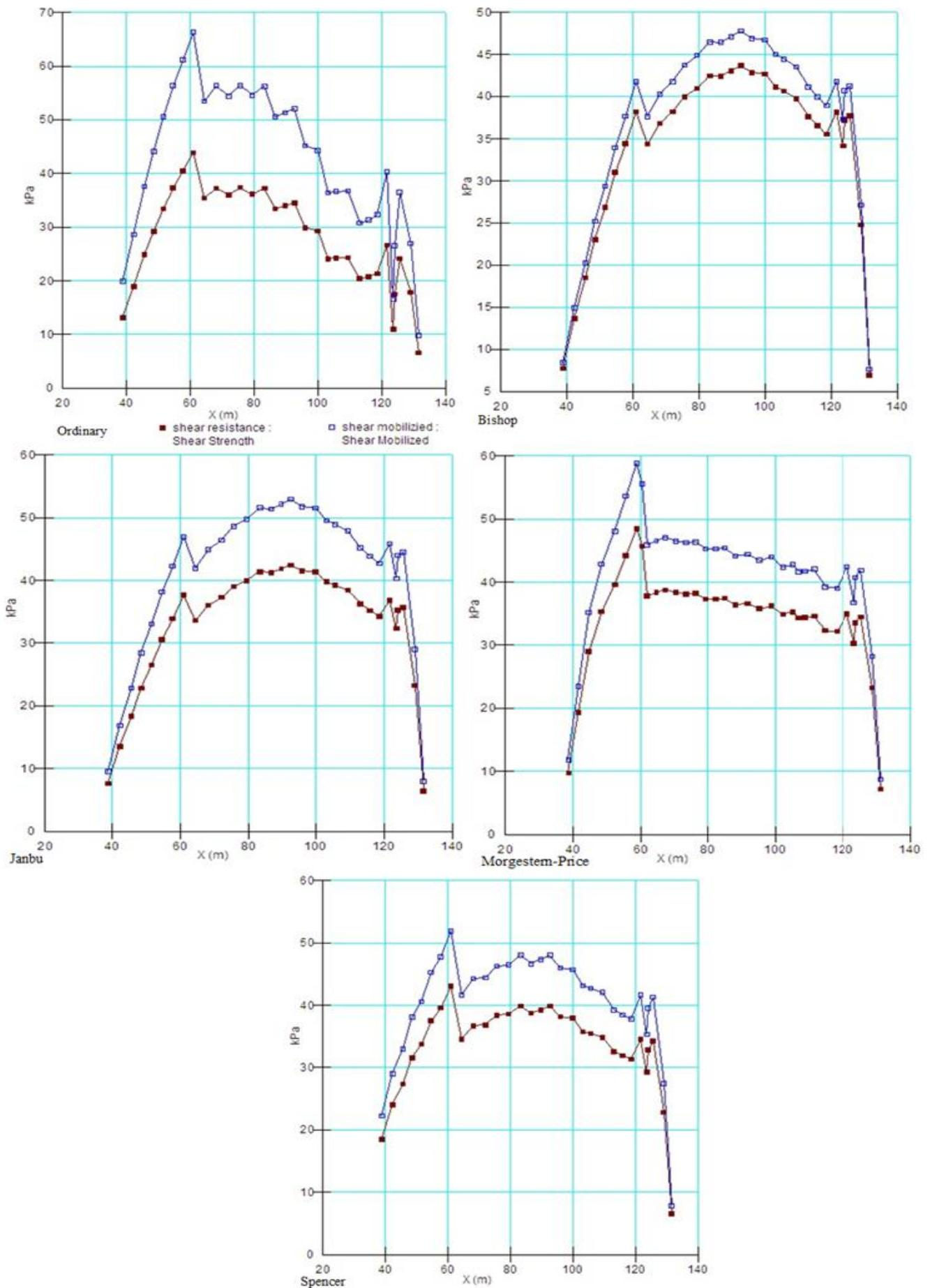
**Figure 10.** Comparison between the driving and the resistance force at the critical failure on earth dams for different ways of Limit Equilibrium Piece
