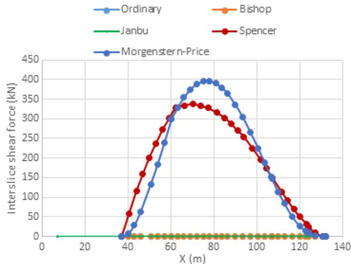
Figure 9. Comparison of the shear inter-piece force to different methods of Limit Equilibrium
