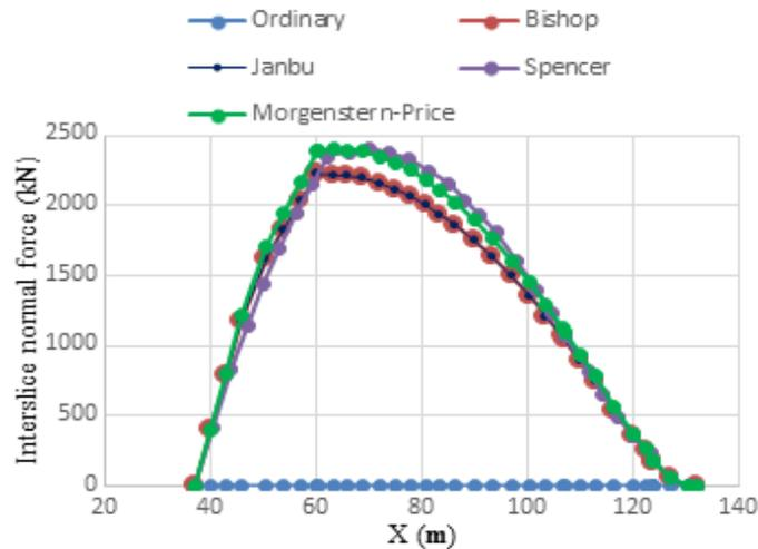
Figure 8. Comparison of the vertical inter-piece force to different methods of Limit Equilibrium
