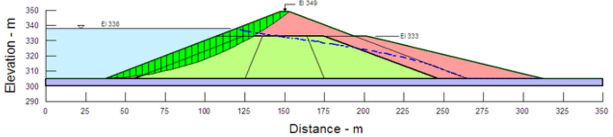
Figure 6. Critical failure surface of earth dams upstream
