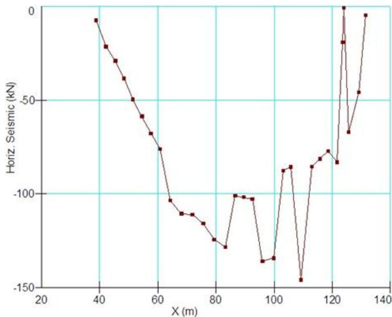
**Figure 13.** Forces due to applied earthquake to the various components
