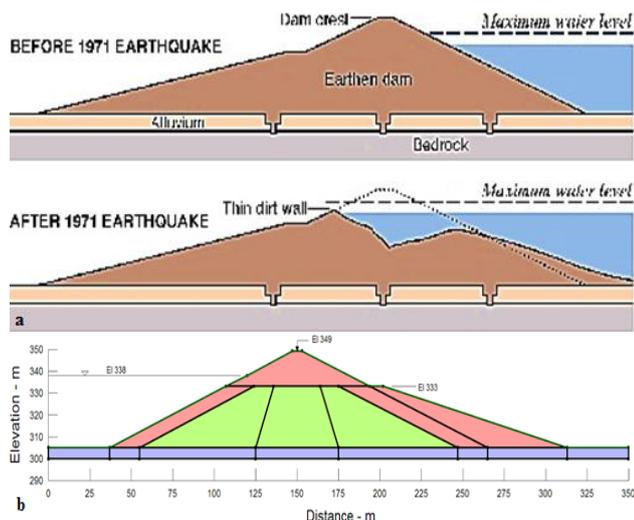
**Figure 5.** (a). Overall view of San Fernando's dam (before and after the earthquake) (Seed, 1975); (b). Modeled earth dam based on San Fernando dam (Seed et al., 1975)
