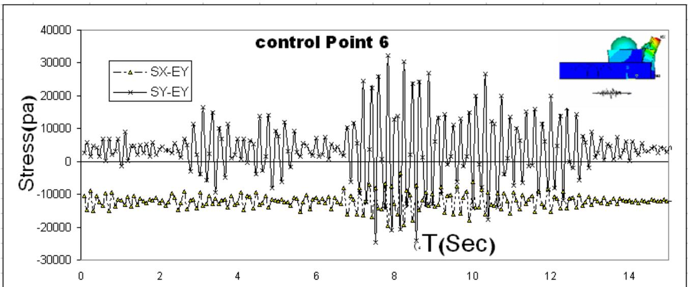
Figure 13. History of stress changes in the control point6 due to seismic stimulation of Manjil earthquake accelerogram
