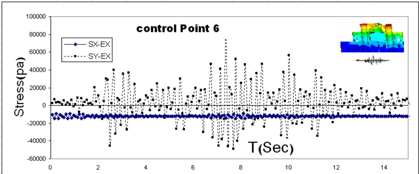
Figure 12. history of stress changes in the control point6 due to seismic stimulation of Manjil earthquake accelerogram
