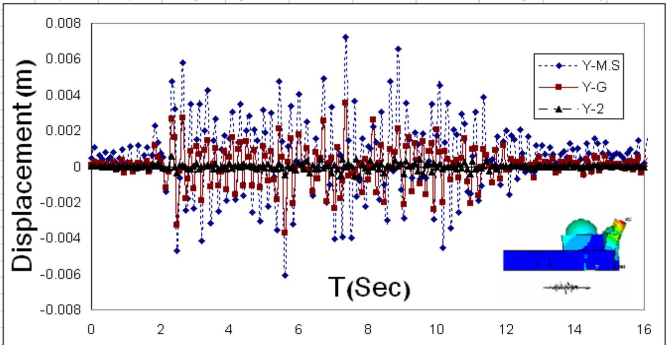
Figure 10. history of control point displacement due to seismic stimulation of Manjil earthquake accelerogram
