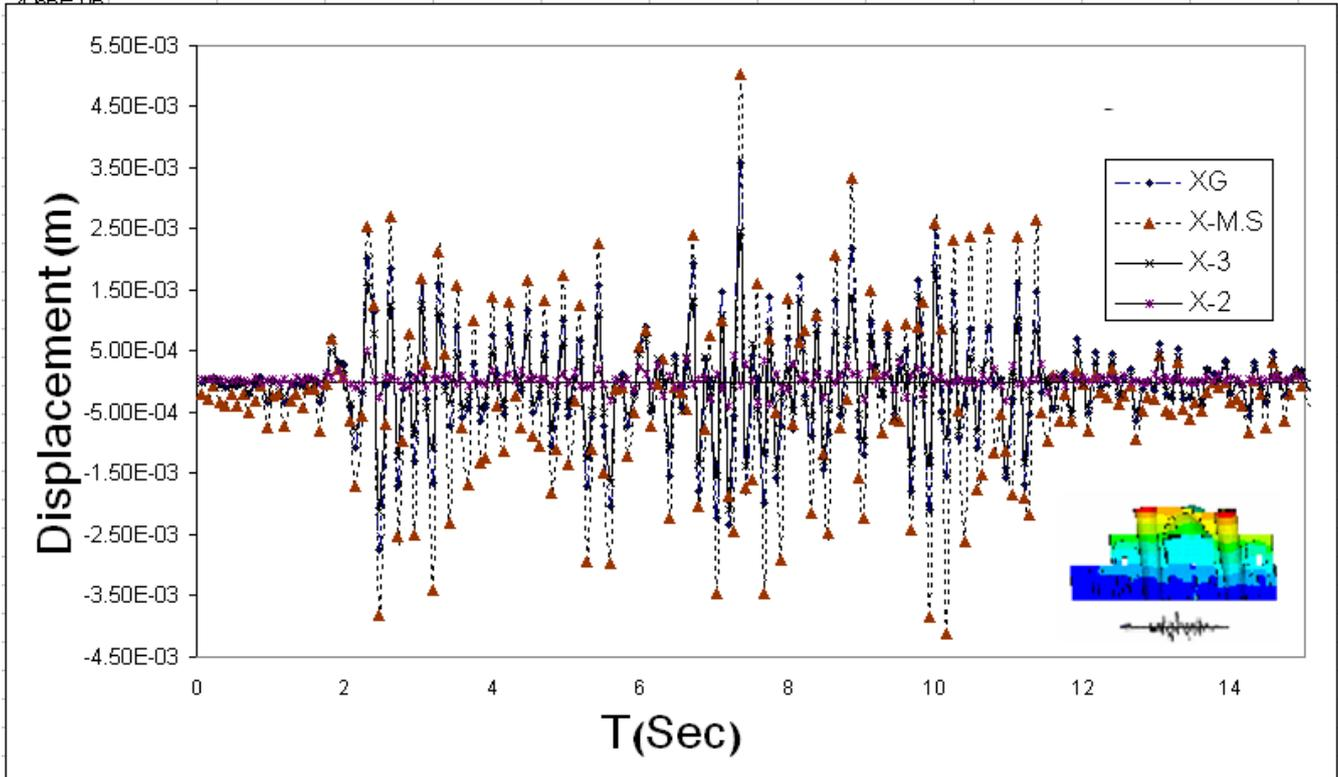
Figure 9. history of control point displacement due to seismic stimulation of Manjil earthquake accelerogram
