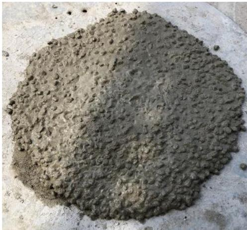
**Figure 2.** Slump flow of developed SCC
