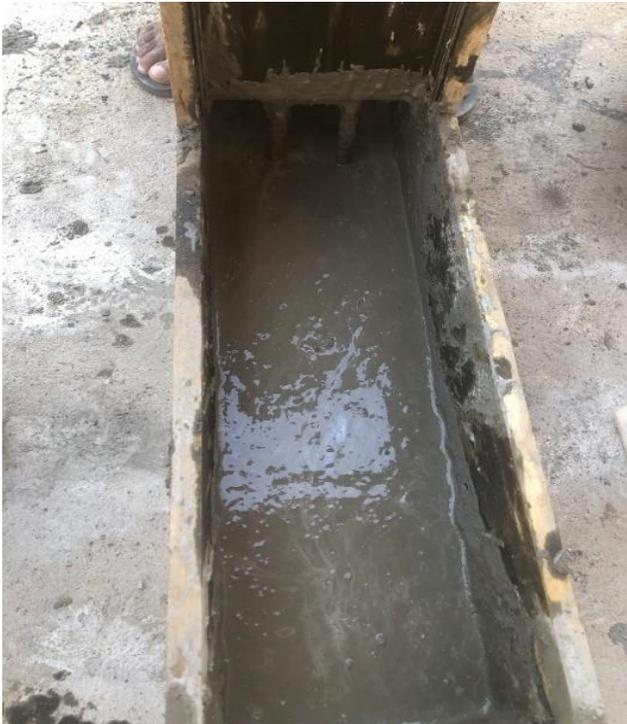
Figure 4 - L- box apparatus with SCC
