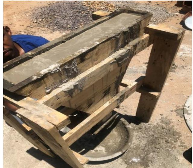
**Figure 3.** V-Funnel apparatus filled with fresh concrete.
