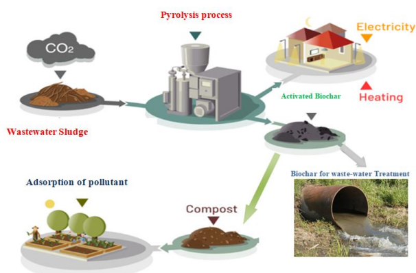
Figure 1. Conversion of Wastewater Sludge to Biochar for electricity, leachates' and soil treatment
