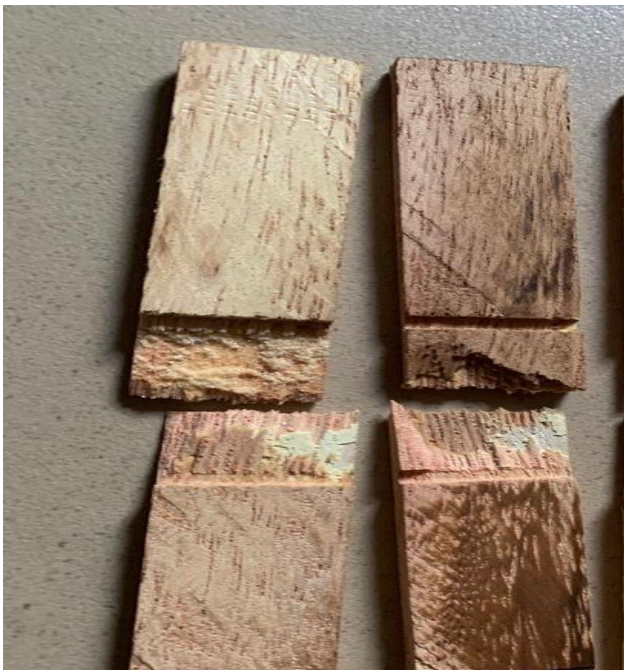
Figure 10b. wood failure in glued joints
