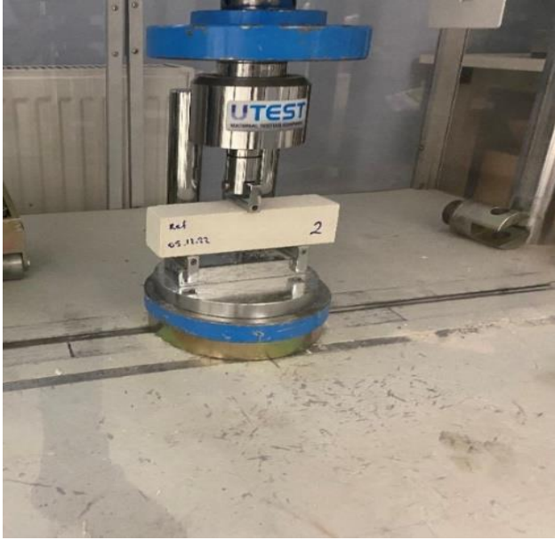
Figure 11. Flexural strength test setup.
