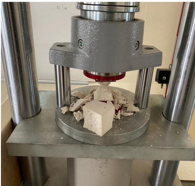
Figure 12. Compressive strength test setup.
