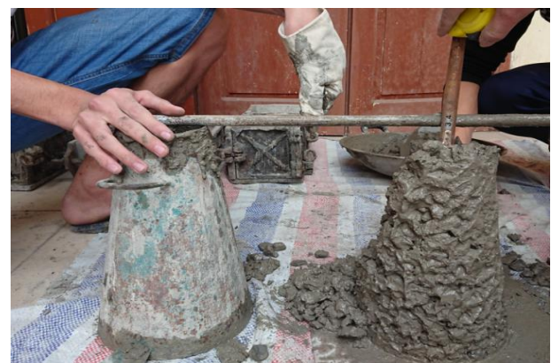
Figure 2. Checking the slump of mixture
