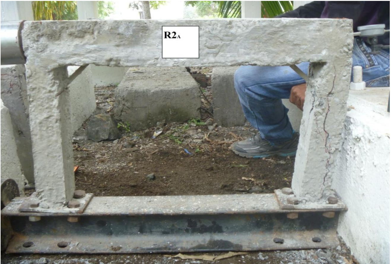
Figure 6. Top corner top bracing R.C. Frame
