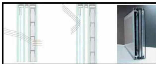
Figure 2. Window section with salt hydrates insulation, summer and winter (Ritter, 2007)
