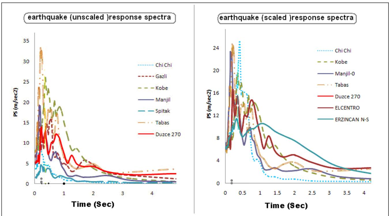
Figure 7. Comparison of selected accelerogram response spectra
