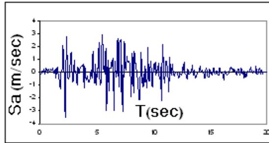
Figure 8. Manjil earthquake accelerogram
