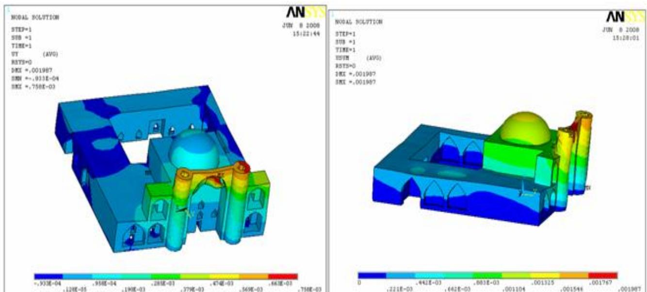
Figure 5. results of model analysis under its own weight
