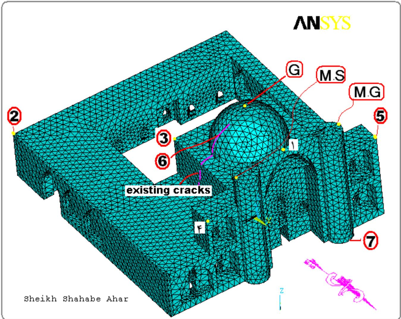
Figure 4. Finite element model of the monuments and introduction of control points
