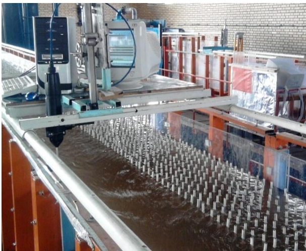
Figure 4. Vegetation array and ADV during data collection
