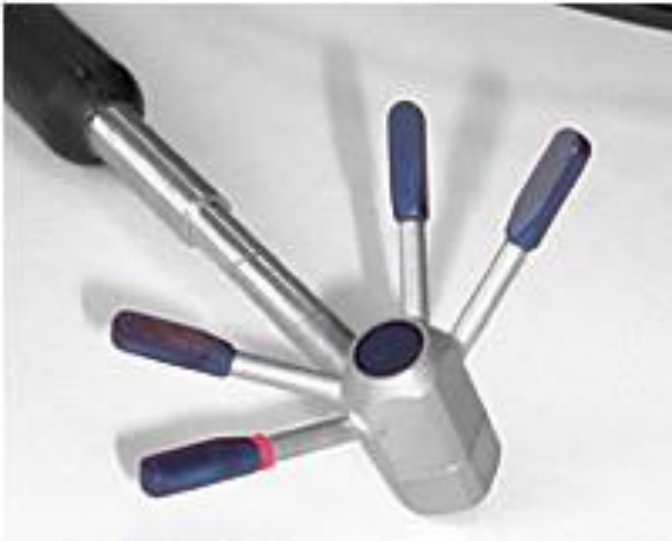
Figure 3. Acoustic Doppler Velocimeter (ADV): a pulse is transmitted from the centre transducer, and the Doppler shift introduced by the reflections from particles suspended in the water, is picked up by the four receivers.
