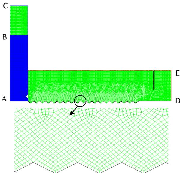
**Figure 2.** Boundary conditions and initial air and water flow regions
